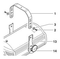
The bracket (1) can also be fitted towards the bottom of the projector. To do this, it is necessary to extract the knobs (14) from the rear hole and turn through 180° both the plates (13) and the spacers (15), then re-insert the knobs (14) into the front hole.
